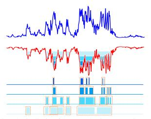
Figure 3. Visualization of the temporal actionness grouping process for proposal generation. **Top**: Actionness probabilities as a 1D signal sequence. **Middle**: The complement signal. We flood it with different levels  $\gamma$ . **Bottom**: Regions obtained by different flooding levels. By merging the regions according to the grouping criterion, we get the final set of proposals (in orange color).
