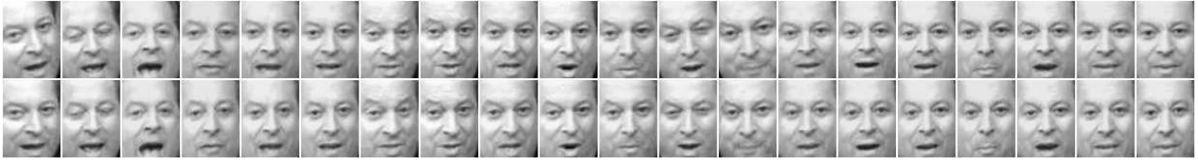
Figure 3: Alignment results of video sequence gore . First row: 20 uniformly sampled frames from the 140-frame gore . Second row: corresponding aligned frames by our method.
