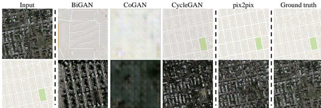
**Figure 5:** Different methods for mapping aerial photos↔maps on Google Maps. From left to right: input, BiGAN/ALI [6, 7], CoGAN [28], CycleGAN (ours), pix2pix [20] trained on paired data, and ground truth.
