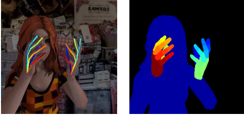
Figure 4: Our new dataset provides segmentation maps with 33 classes: three for each finger, palm, person, and background. The 3D kinematic model of the hand provides 21 keypoints per hand: 4 keypoints per finger and one keypoint close to the wrist.
