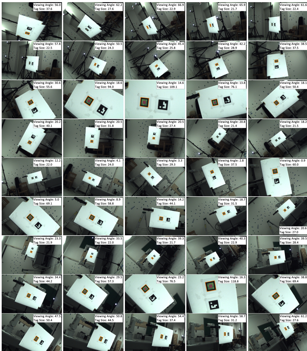
Figure 3: Example images processed by ChromaTag with labeled tag size and viewing angle.
