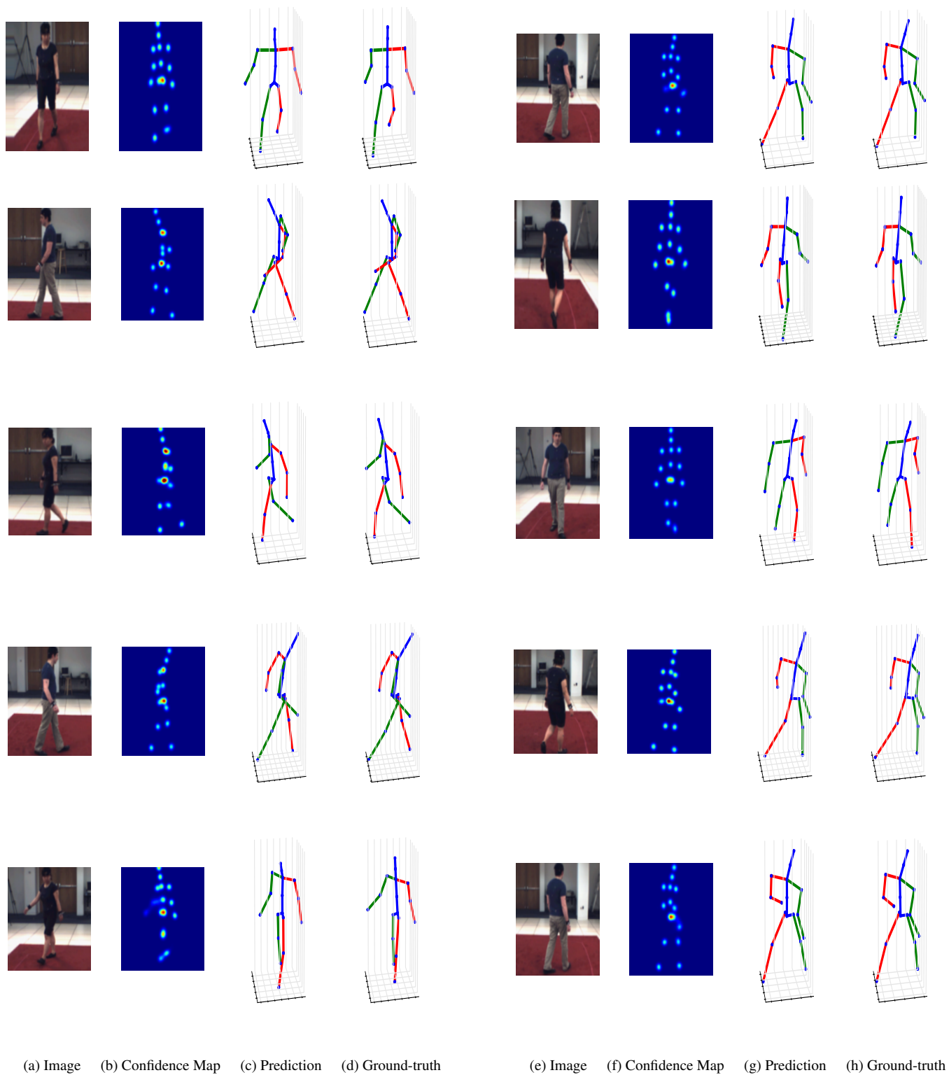
Figure 3. Pose estimation results on HumanEva-I. (a, e) Input images. (b, f) 2D joint location confidence maps. (c, g) Recovered pose. (d, h) Ground truth. Best viewed in color.
