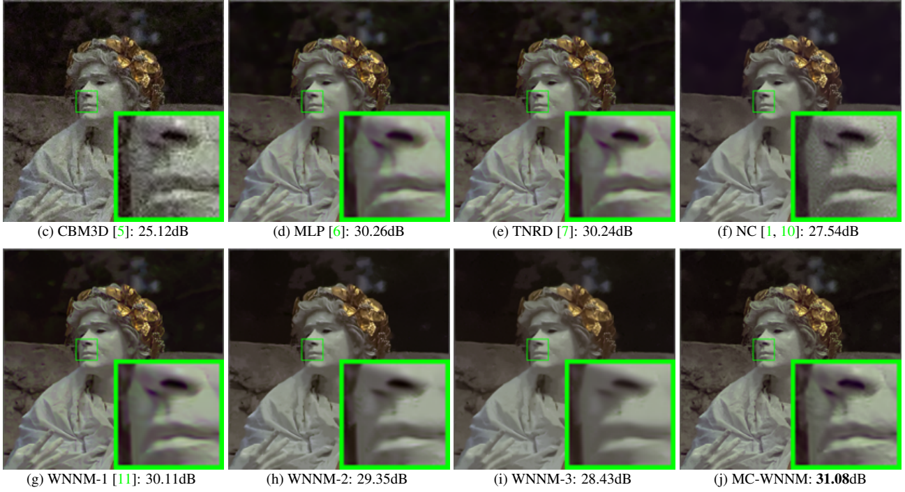
Figure 3. Denoised images of different methods on the image “kodim17” degraded by AWGN with different standard deviations of \sigma_r = 30, \sigma_g = 10, \sigma_b = 50 on R, G, B channels, respectively. The images are better to be zoomed in on screen.
