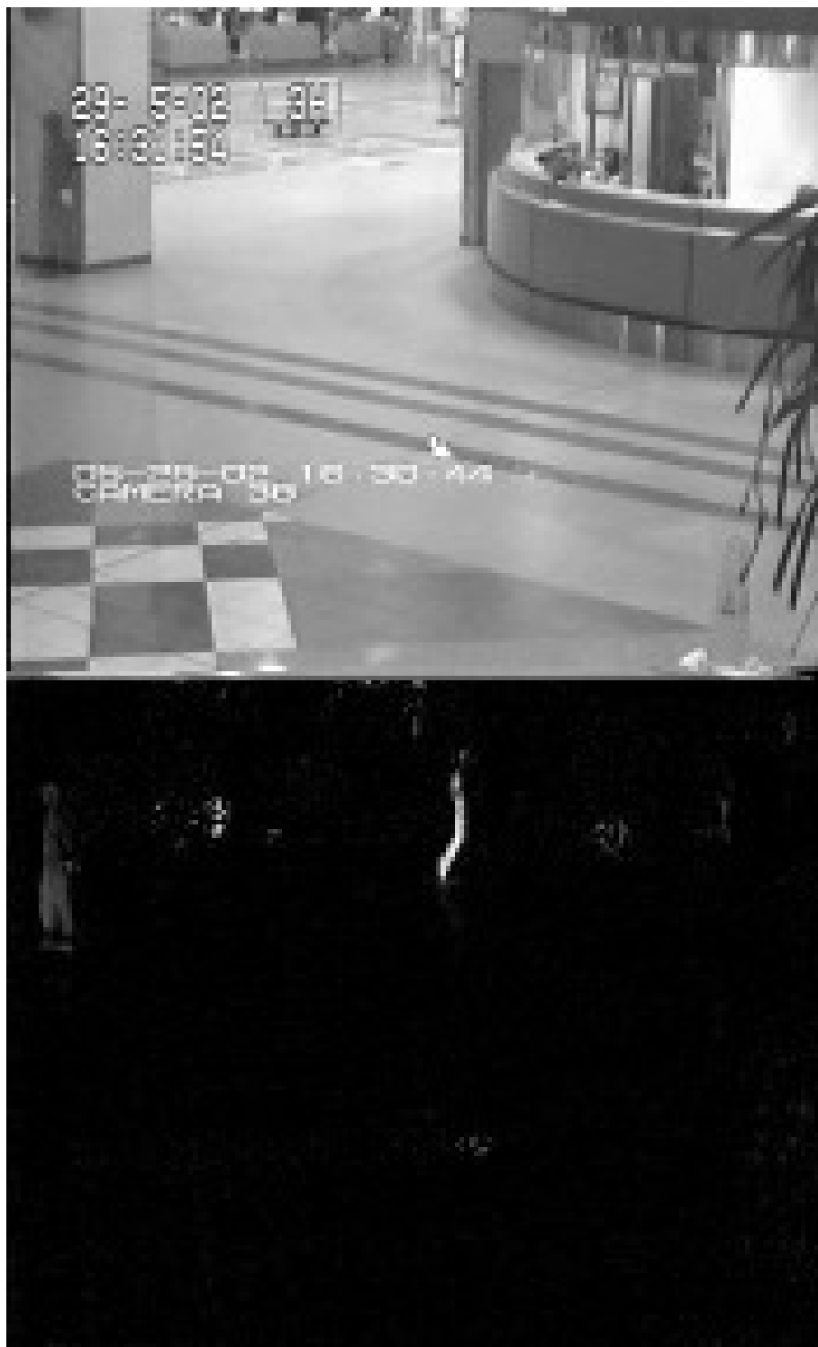
Figure 9: Background subtraction by suggestion: background in row I and segmentaion in row II .
