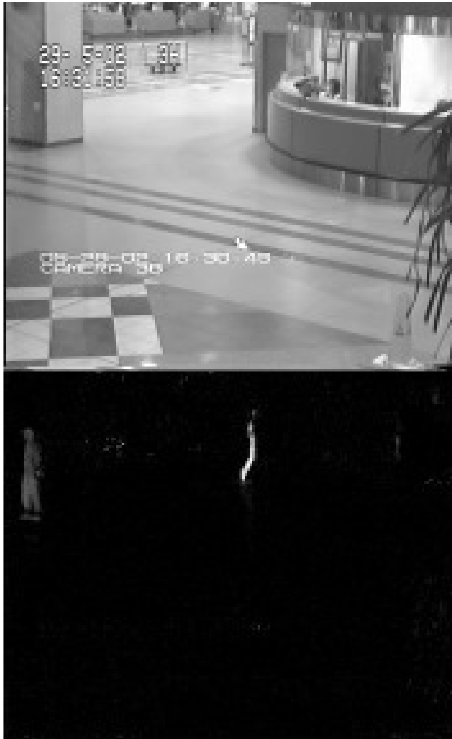
Figure 10: Background subtraction by PCPS: background in row I and segmentation in row II .
