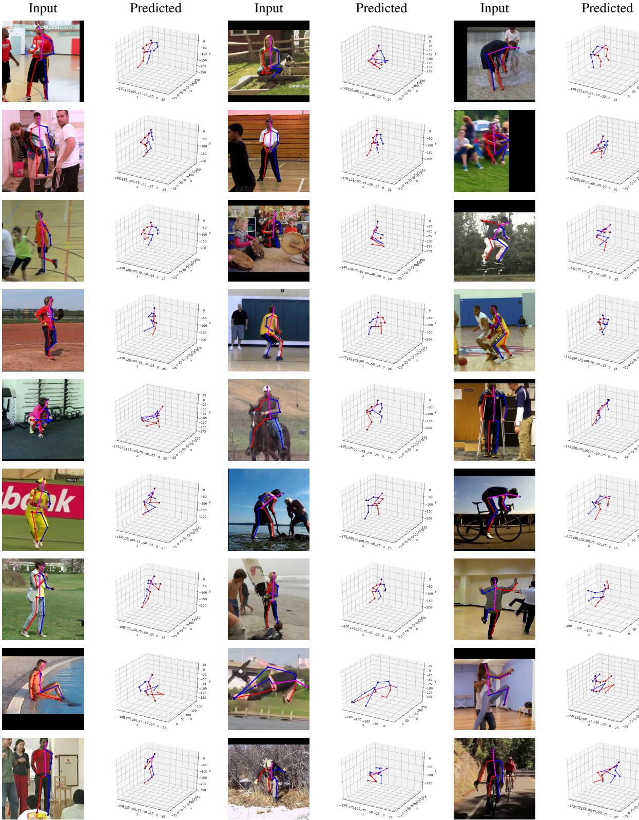
Table 1. Qualitative results from MPII validation sets. We show our predicted poses. Our framework performs well in a wide range of poses and situations. Typical failure cases (the last two lines) include inaccurate 2D prediction and ambiguous depth.
