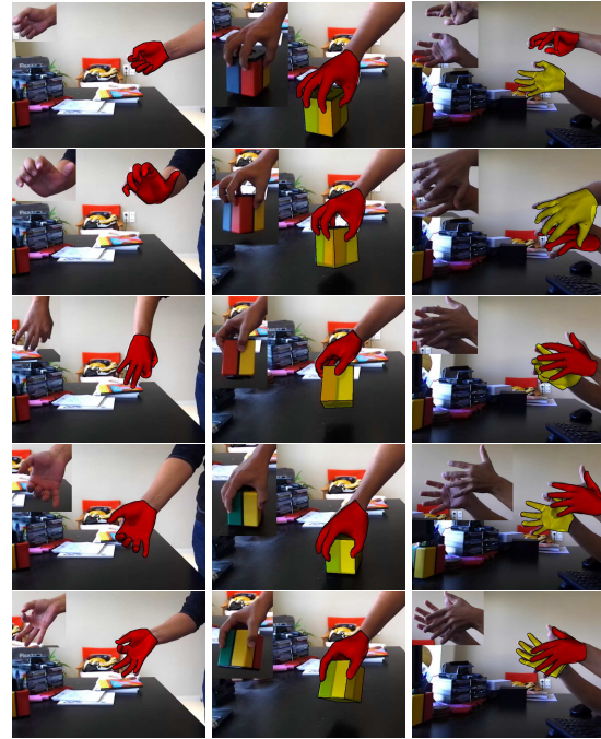
Figure 5. Qualitative evaluation. Results on real world sequences. Tracking of a single hand sequence (left), of a hand interacting with a pencil box (middle) and of two interacting hands (right).
