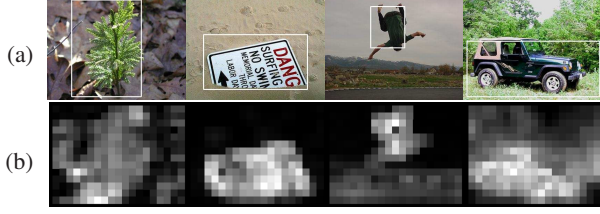
Figure 3. (a) Example images from the MSRA dataset, rectangles showing the regions extracted based on Dmap, (b) the Dmap feature maps.
