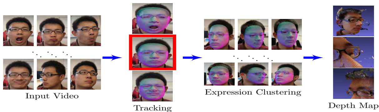
Figure 1: Given a video, a parametric 3D model [6] was fitted to noisy 2D landmarks produced from the off-the-shelf 2D landmark detector[21]. The fitted 3D model is used to refine the 3D position computed from the 2D landmarks via robust photometric tracking. The tracked 3D mesh are superimposed on the image. After clustering, video frames of similar facial expressions as seen at different viewing angles are used to compute a complete and smooth dense depth map. The glasses and hair are well reconstructed.
