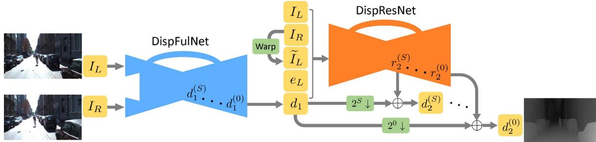
Figure 1. Network architecture of our *cascade residual learning* (CRL) scheme. The first stage is *DispFulNet* and the second stage is *DispResNet* with multiscale residual learning. The module “ $2^s \downarrow$ ” is the downsampling layer to shrink  $d_1$  for  $2^s$  times, while “Warp” denotes the warping layer.
