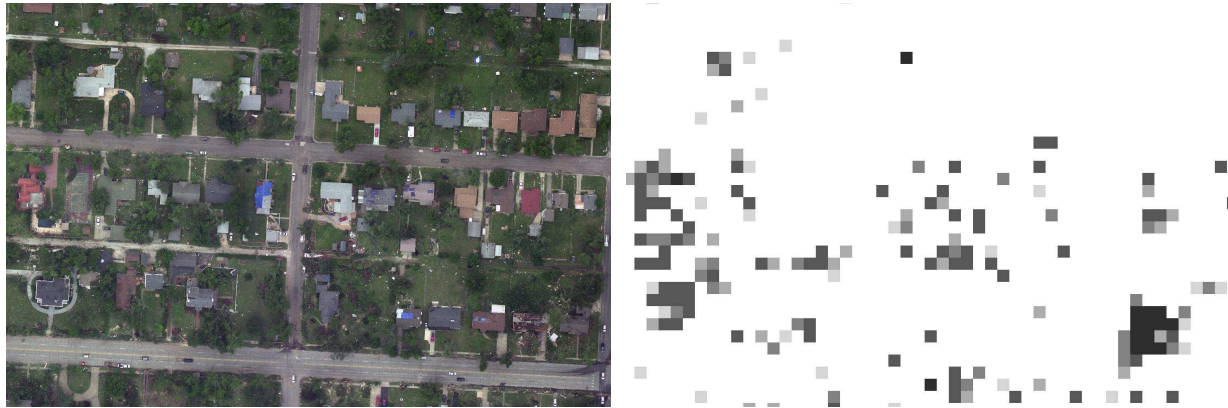
Figure 6. Figure, in the right-hand side, shows the amount of processing (number of stages used in the cascade) in order to reject or accept different patches in the test image (shown in the left-hand side); darker colors correspond to more intense processing.
