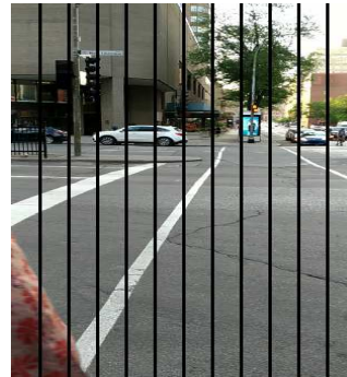
Figure 1: Action space discretization into vertical bins \mathcal{V} = \{v_1, \dots, v_{12}\} from left to right.
