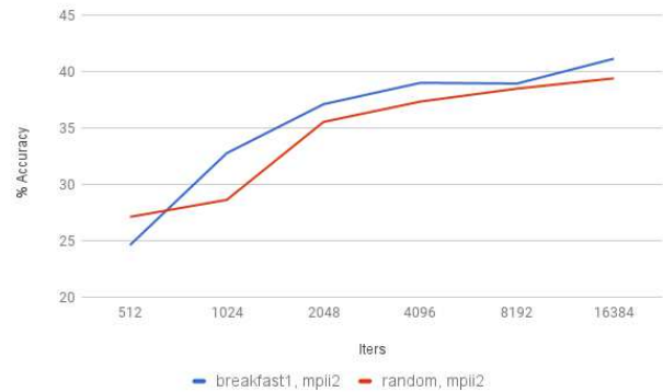
Figure 5: Convergence on split 2 of the MPII Cooking 2 dataset when pre-trained with other datasets and random initial weights.
