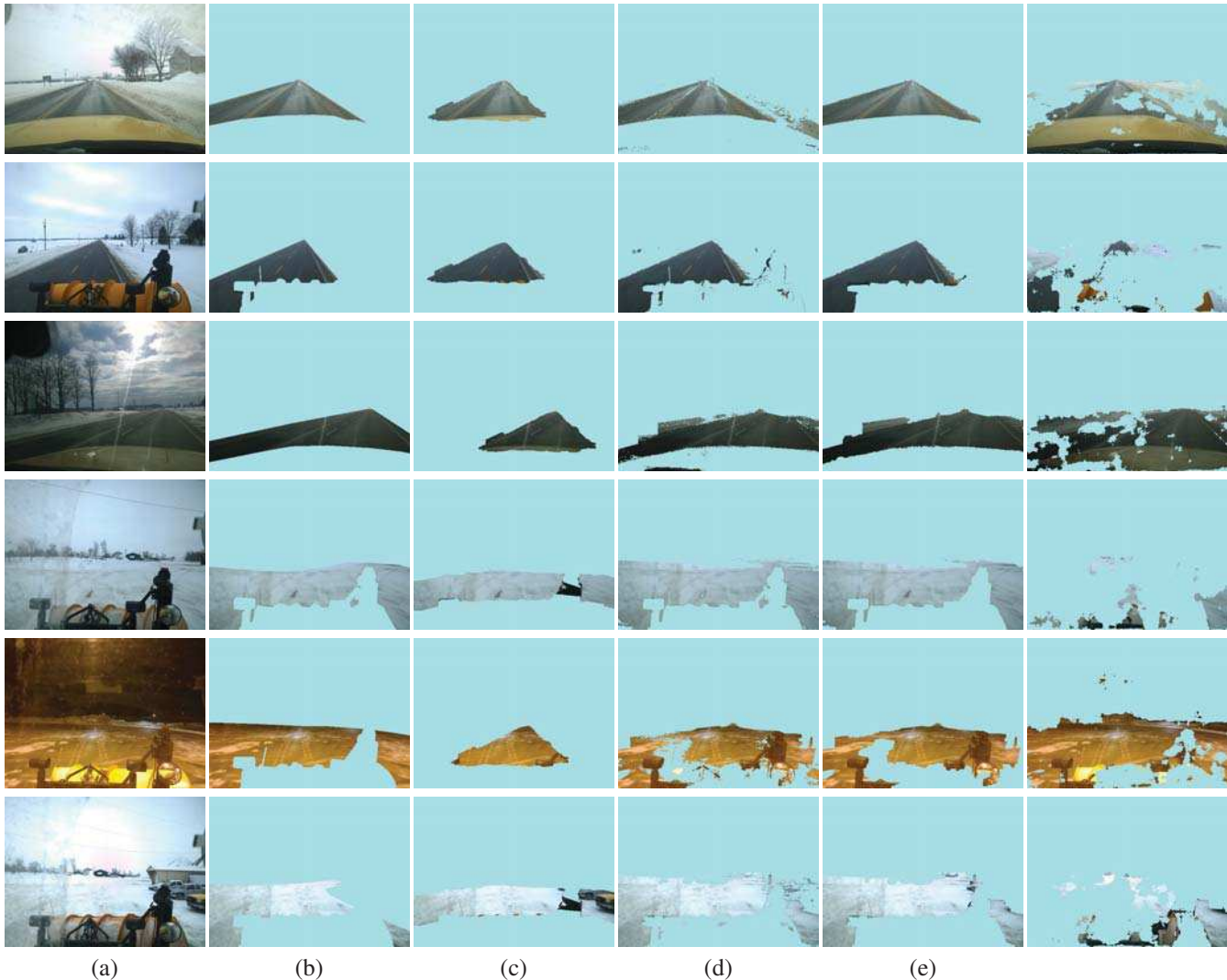
Figure 8. Example results. (a) Test image (b) Ground truth segmentation. (c) Geometric method [1]. (d) Fusion method (initial). (e) Fusion method (refined). (f) SegNet method (road + pavement)
