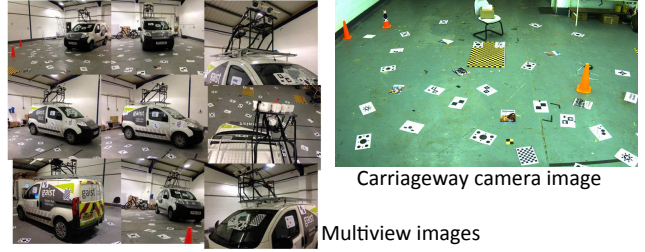
Figure 3. Left: Subset of the multiview images used to reconstruct the capture vehicle model. Right: image from the carriageway camera also used in the reconstruction.
