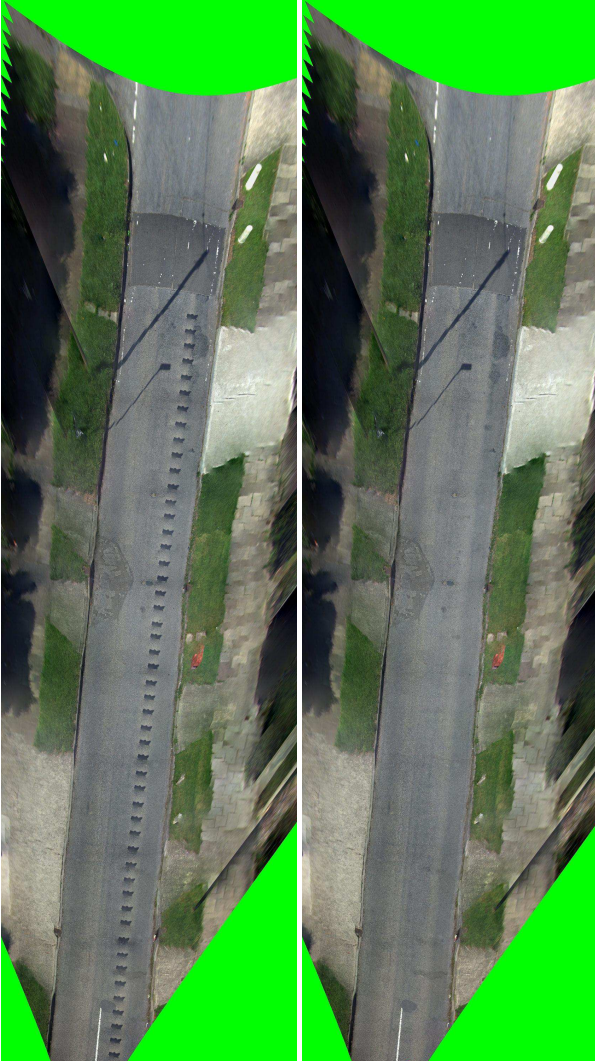
Figure 7. Stitching results on a 50 image sequence. Left: results without shadow modelling (note repeated shadow pattern). Right: result with shadow-aware weights (shadow pattern is completely eliminated yet stitched result remains seamless).
