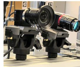
Figure 3: Hyperspectral cameras used to capture the new datasets.
