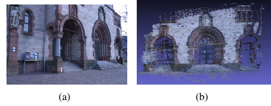
Figure 7: (a) Original 2D image, (b) dense 3D point cloud estimated with D-ADMM BA (mean re-proj. error = 0.76).
