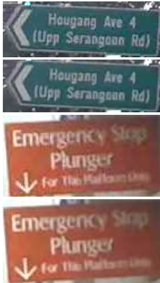
Figure 1: Examples of compression artifact removal. Odd rows: compressed images with compression artifacts; even rows: results of the proposed system. Best viewed in color and zoomed in.
