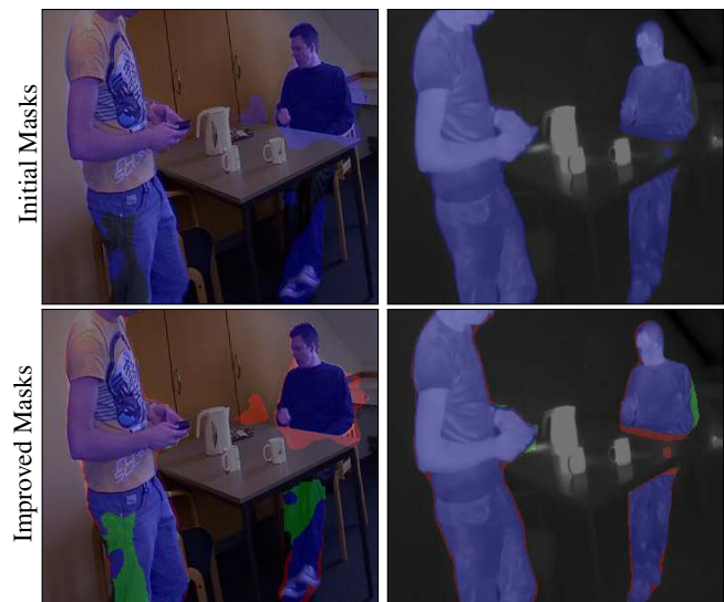
Figure 1. Example of mutual foreground segmentation improvement for a visible-LWIR stereo pair. The initial foreground masks obtained via background subtraction are shown in the top row as regions highlighted in blue. These are refined almost ideally using our proposed approach in the bottom row, where green shows added foreground pixels, and red removed foreground pixels.
