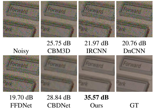
Figure 9. A challenging example from SSID dataset [1]. Our method can remove noise and restore true colors.
