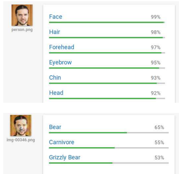
Figure 5. Adversarial image (target "bear"), classified by Google Cloud Vision after 346 queries. Confidence scores are displayed, but not used by the attack. No label hinting at a person is left (the prediction vector contains only 3 labels).
