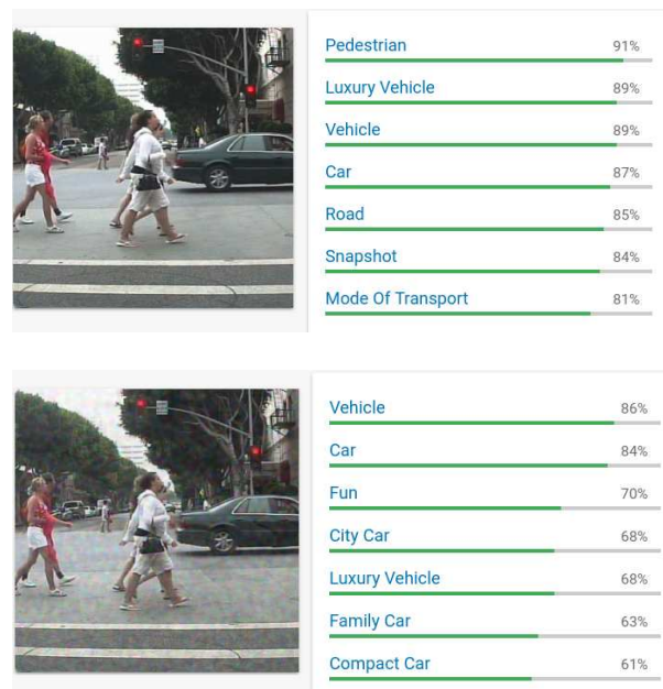
Figure 6. Adversarial image (pedestrians have been removed), classified by Google Cloud Vision after exactly 1000 queries. Confidence scores are displayed, but not used by the attack. Perhaps interestingly, our adversarial pattern is classified as "Fun".
