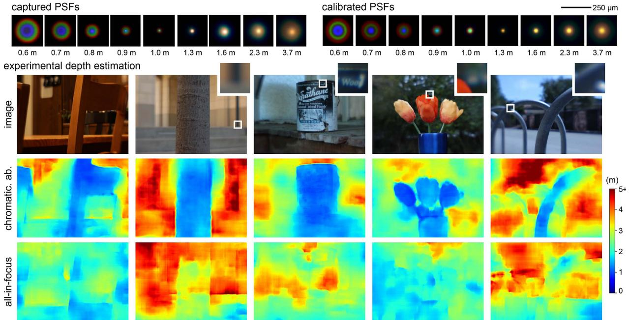
Figure 5. **Real-world capture and depth estimation.** (Top) Captured and calibrated depth-dependent PSFs, displayed at the same scale. (Bottom) Examples of images captured using our prototype with a zoomed region inset, depth estimation with chromatic aberration, and depth estimation from the corresponding all-in-focus image (not shown). Depth map colorscale is the same for all depth maps.
