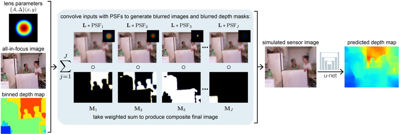
Figure 3. **Depth-dependent image formation.** Given a set of lens parameters, an all-in-focus image, and its binned depth map, the image formation model generates the appropriate PSFs and applies depth-dependent convolution with masking to simulate the corresponding sensor image, which is then passed into a U-Net for depth estimation.
