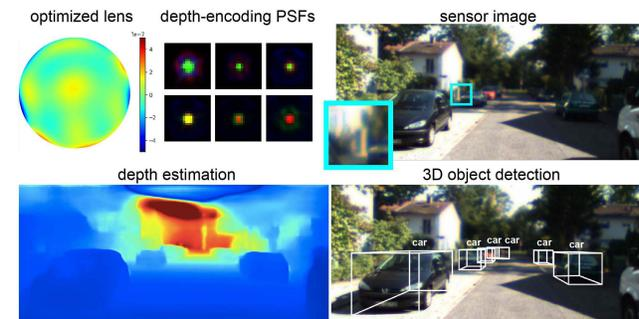
Figure 1. We apply deep optics, i.e. end-to-end design of optics and image processing, to build an optical-encoder, CNN-decoder system for improved monocular depth estimation and 3D object detection.
