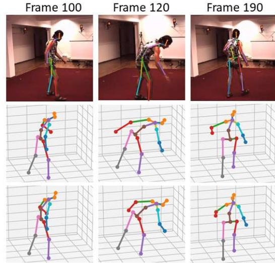
Figure 5. Example of the effectiveness of pose regularization. The second row shows wrong 3D estimation without the regularization term. The third row shows that the constraint fixes the error.
