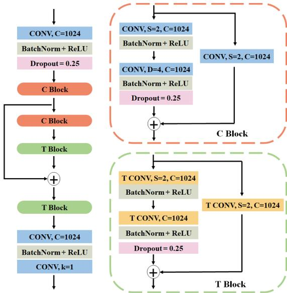
Figure 6. Illustration of our temporal convolutional network structure. *CONV* and *T CONV* stand for convolutional and transpose convolutional operations. *S*, *C*, and *D* stand for stride, channel and dilation rate, respectively. The kernel size for all blocks are set to 5.
