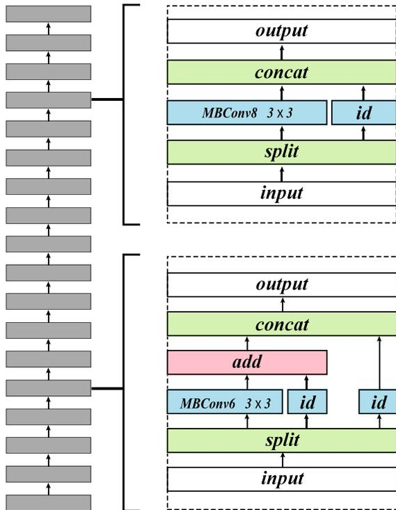
Figure 5. More details of our searched network structure. Blocks at different positions are with their special topological architectures. *MBCConv6* and *MBCConv8* are mobile inverted bottleneck convolution with expansion ratios 6 and 8 respectively.
