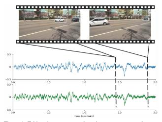
Figure 1. Taking the stereo sounds as input, our proposed crossmodal auditory localization system can recover the coordinates of moving vehicles in the reference frame purely from stereo sound and camera meta-data, without any visual input.
