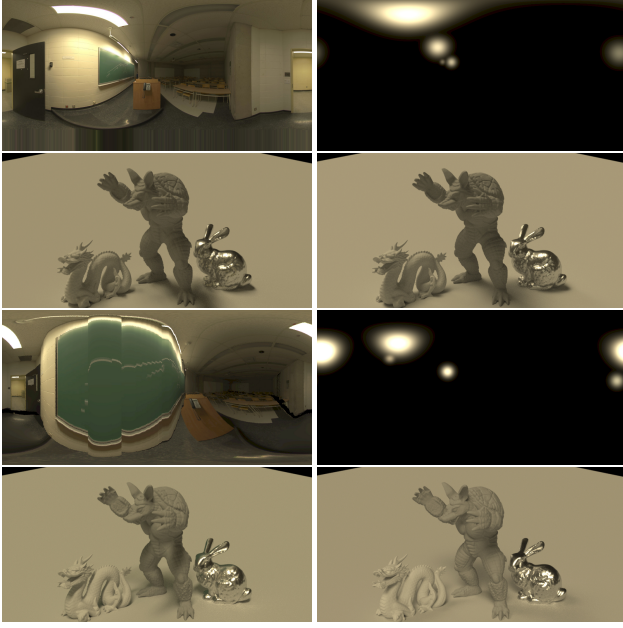
Figure 2. Comparison between an environment map and our lighting representation for relighting. Top row: source HDR panorama, and spherical gaussian representation of the parameters. Second row: renders generated by both representations. Third and fourth row: lighting and renders when moving in the scene, using EnvyDepth [1] as ground truth. Note how our parametric lights stay true to the ground truth for a different location in the scene.
