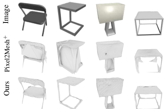
Figure 6. Pixel2Mesh + predicts meshes by deforming an initial sphere, so it cannot properly model objects with holes. In contrast our method can model objects with arbitrary topologies.
