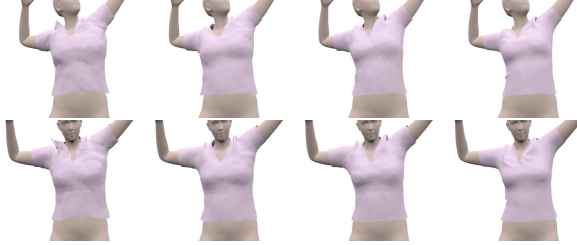
GarNet-Naive GarNet-Global GarNet-Local PBS Figure 8: Comparison on the T-shirt. GarNet-Naive produces artifacts near the shoulder while GarNet-Local, GarNet-Global and PBS yield similar results.
