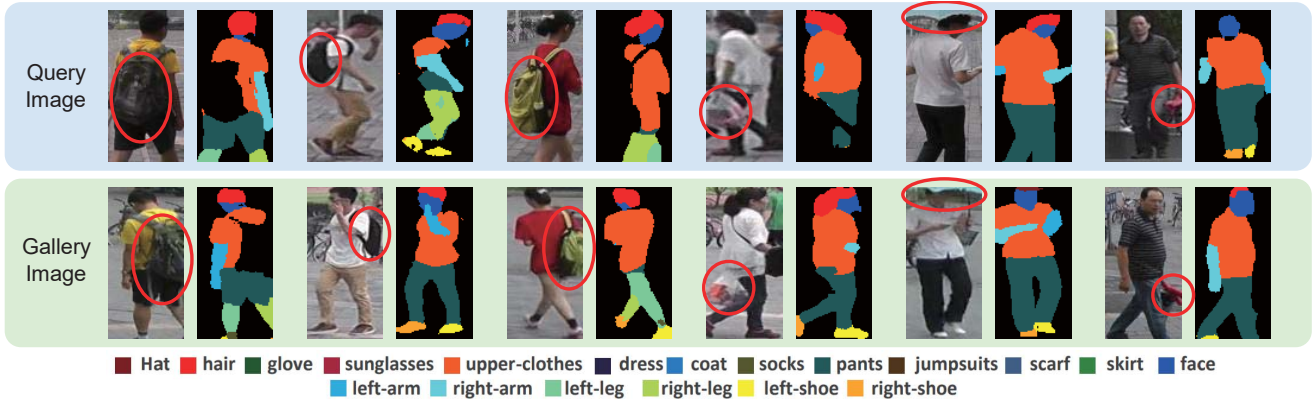
Figure 1: Failure cases of the human parsing model: The first row illustrates the query images, the second row illustrates the gallery images from Market-1501 and each column consists of two images belonging to the same identity. All of the regions marked with red circle are mis-classified as background (marked with black color) due to the limited label set while their ground-truth labels should be backpack, reticule and umbrella. It can be seen that these mis-classified regions are crucial for the person re-identification.
