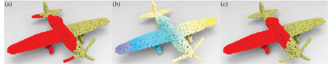
Figure 3. The comparison of front halves (red parts in (a) and (c)) split by Euclidean distance and geodesic distance (map in (b)).
