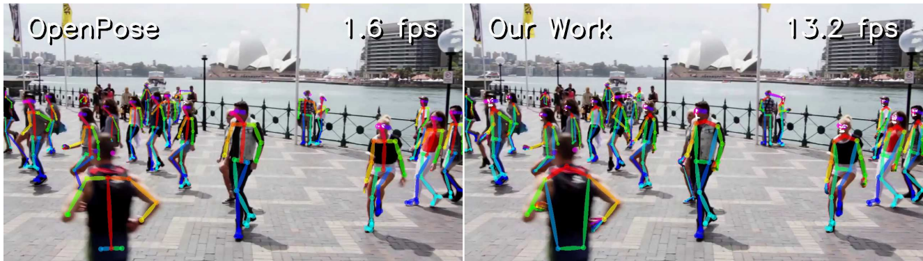
Figure 1: We present the first single-network approach for whole-body pose estimation, with real-time performance independent of the number of people in the image. Our work builds upon the current state-of-the-art OpenPose [9], boosting considerably its run-time performance while simultaneously improving slightly on the keypoint accuracy.
