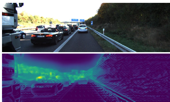
Figure 1. An example of the proposed visualization of single view depth estimation. Upper: an input image. Lower: a mask generated by our method showing relevant pixels for depth estimation.
