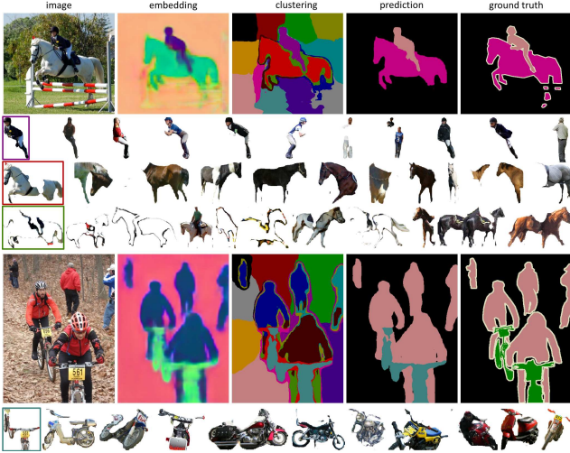
Figure 5. Two examples, correct and incorrect predictions, for segment retrieval for supervised semantic segmentation on VOC 2012 validation set. Query segments (leftmost) are framed by the same color in clustering. (Top) The query segments of rider, horse, and horse outlines can retrieve corresponding semantically relevant segments in the training set. (Bottom) For the failure case, it can be inferred from the retrieved segments that the number tag on the front of bikes is confused by the other number tags or front lights on motorbikes, resulting in false predictions.
