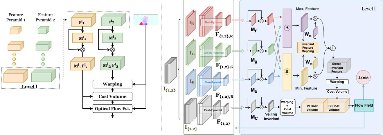
Figure 2: Left: Detailed structure for extracting the feature multiplier  $M$  when computing optical flow at each pyramidal level. Right: the architecture for the full solution. Layer  $A$  and  $B$  are global maximum and global minimum operation respectively. VI stands for veiling-invariant, and SI stands for streak-invariant.
