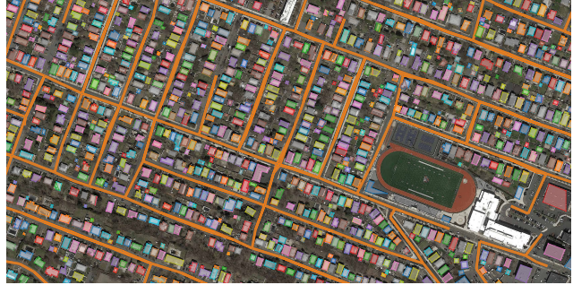
Figure 1: PolyMapper result for Boston overlaid on top of the original aerial imagery. Buildings and roads are directly predicted as polygons. See additional results in Fig. 10.
