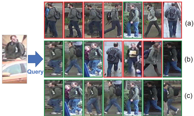
Figure 3. A retrieval example on DukeMTMC-reID. (a) is the result of the model with classification branch only. (b) is generated by the proposed model ( i.e. SFT + classification). (c) is the refined result based on (b) using local blurring re-ranking.
