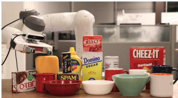
Figure 10. Each object is evaluated on three different poses. The 3D models of these objects are unknown. The training data consists of mugs, bowls, boxes, cylinder, and bottles with random scales. See the supplements for videos of the grasping trials.
