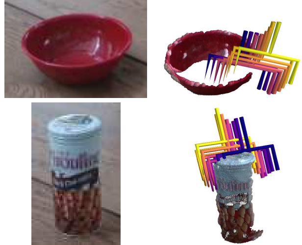
Figure 5. Iterative Grasp Refinement: (left) Image of the object. (right) Grasps colored according to refinement iteration. Dark blue are grasps initially generated from the VAE and yellow are final, refined grasps. Note that even though there are no points between the gripper fingers for the initial bowl grasp (blue), the evaluation network is able to push the gripper to a successful grasp pose.
