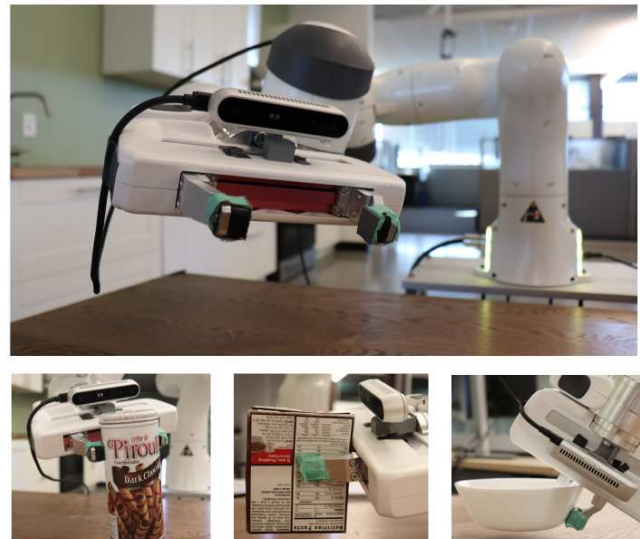
Figure 1. The Franka Panda manipulator used in our experiments. Our approach is able to efficiently generate diverse sets of grasps that lead to successful pickups of unknown objects.
