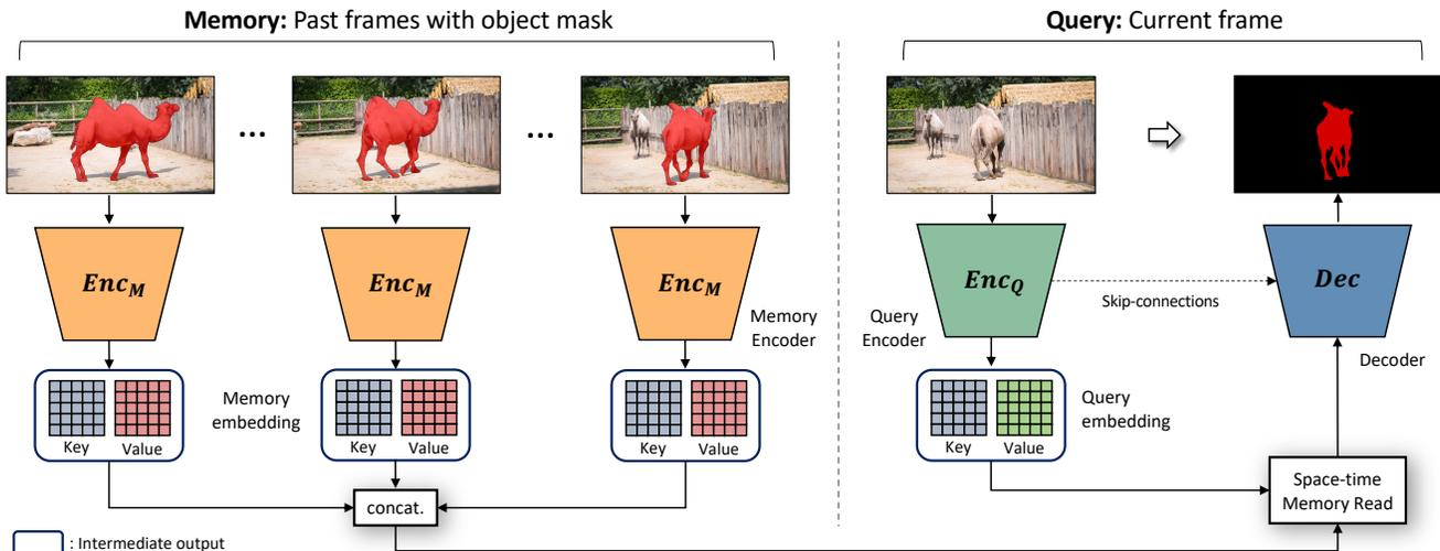
Figure 2: Overview of our framework. Our network consists of two encoders each for the memory and the query frame, a space-time memory read block, and a decoder. The memory encoder ( $Enc_M$ ) takes an RGB frame and the object mask. The object mask is represented as a probability map (the softmax output is used for estimated object masks). The query encoder ( $Enc_Q$ ) takes the query image as input.
