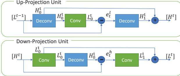
Figure 5. The up-projection and down-projection units in DBPN.
