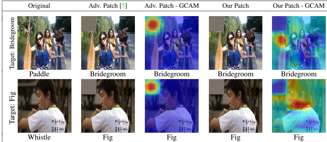
Figure 2: Targeted patch attack: We use an ImageNet pretrained VGG 19 BN network to compare the Grad-CAM visualization results for a random target category using our method vs Adv. Patch [5]. The predicted label is written under each image. Note that the patch is not highlighted in the last column.
