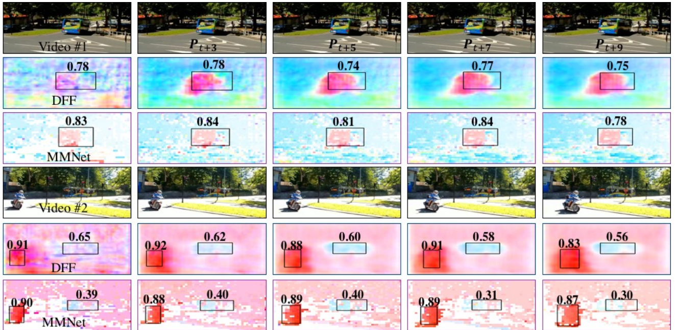
Figure 6. Visualization of FlowNet and Motion Vector. The FlowNet in [54] is capable of building detailed model information. And the motion vector can quickly provide the motion cues which helps to speed up detection procedure in most situations.
