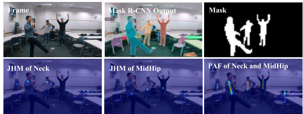
Figure 5. Example of annotations from a video frame: body segmentation mask computed by Mask R-CNN [20], JHMs and PAFs computed by OpenPose [9].
