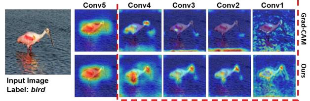
Figure 5. The comparison of attention maps from different VGG-19 [33] layers. Ours has less attention shift than Grad-CAM [31]. In the marked areas, ours attends to the target objects, *i.e.* bird, while Grad-CAM [31] tends to highlight the background pixels.
