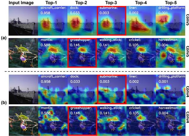
Figure 2. Grad-CAM [31] attention maps of the VGG-19 [33] top-5 predictions. Predictions with red-bounding boxes correspond to the ground-truth class. (a) Ground-truth class attention maps from the last layer (Conv5) have a large overlap with false positives (top-1 predictions). (b) Inner-layer attention maps (Conv4) are more separable than their last-layer counterparts.
