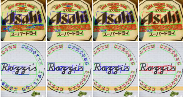
Figure 3: Character bounding boxes generated at 4 interactive steps from left to right. Red boxes indicate the identified “correct” ones by our rule, while blue boxes mean invalid ones, which are not collected for training in next step.
