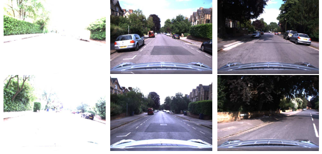
Figure 6: Samples of challenging conditions on the RobotCar dataset [19]. From left to right: three pairs of images demonstrate the observations with over-exposure, changing weather and dynamic objects, similar appearances at different locations.
