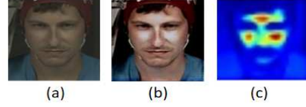
Figure 8. Visualization of model output images. (a) face image in compressed video; (b) STVEN enhanced face image; (c) rPPGNet predicted attention map.
