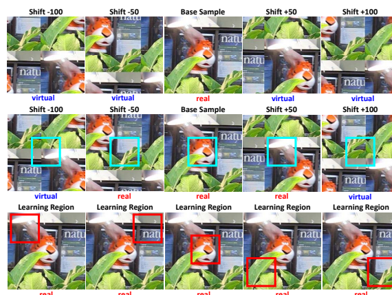
Figure 1: Comparison of sampling methods in KCF [22] (1st row), BACF [24] (2nd row), and our fdKCF* (last row). Training samples of KCF come from the cyclic shift of a base sample (i.e. learning region), and they are all virtual except for the base one. BACF obtains its training samples with target size (cyan boxes) by clipping the middle parts of all training samples of KCF, and some of them are virtual. Different from them, in fdKCF* , training samples with target size (red boxes) are densely sampled from the learning region in the traditional sliding window way, and they are all real. We call our sampling method as real and dense sampling .
